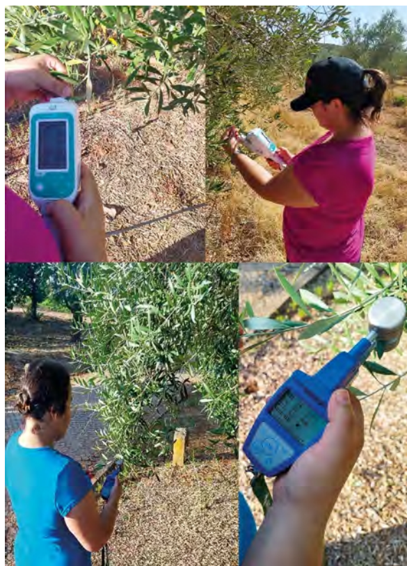
Figure 10 – Non-destructive measurements using the LI-600 porometer/fluorometer (top) and the Dualex (bottom) on olive leaves ( Olea europaea L.)
